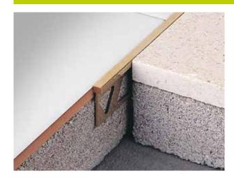
LINETEC MB decorative profiles are installed on site in mortar bed applications. Its perforated flange deeply inserted into the mortar guarantees a secure grip between the two adjacent surfaces. It is commonly used with natural stone flooring to decoratively segment the floor surface. Available in brass and aluminum, both the 5mm and 10mm profile widths can be ground and polished on site.
